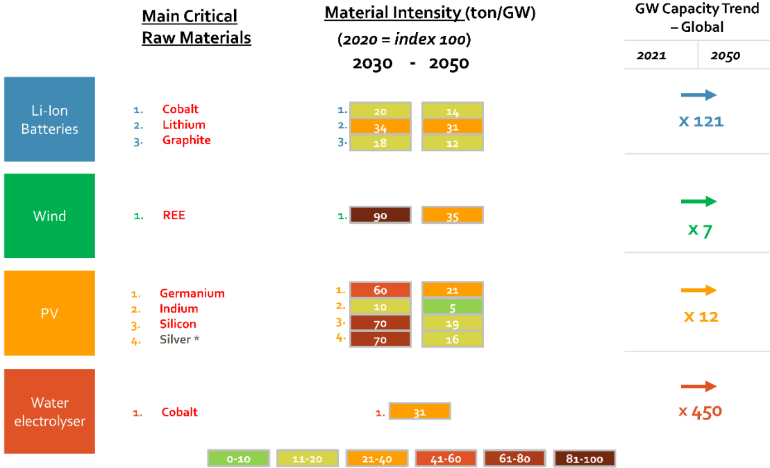
Figure 5 Material efficiency for a selection of CRM between 2020 and 2050 (2040 in case of electrolyzers) expressed in tons of material used per GW of manufactured asset (European Commission, 2020) compared to the foreseen increase in installed capacity required to meet our climate ambitions (IEA, 2022). (The asterisk (*) indicates that silver is not listed as CRM in the 2023 list of EU CRM (European Commission 2023) but is still included due to its important role and related cost in the production of silicon-based PV panels)
